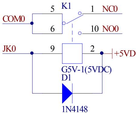
In normal, the relay is OFF, there is contact between the COM post and NC post.
