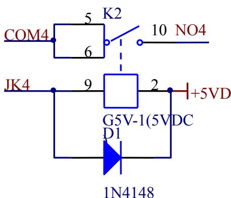
When select the relay 4 is ON, there is contact between the COM4 post and NO4 post. If select the relay 4 is OFF, there is contact between the COM4 post and NC4 post.
