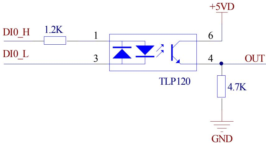
When DI0\_L is ground, DI0\_H inputs high-level, the opto-coupler turns on, the output signal OUT is high-level; DI0\_H input low-level, the opto-coupler does not turn on, the OUT is low-level.
